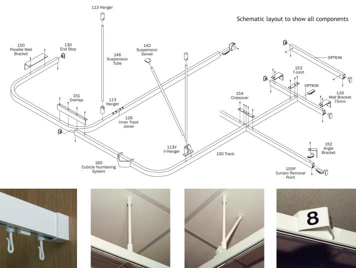
Die-cast aluminium wall shoe, press-slide curtain removal point, and roller wheel curtain hooks
