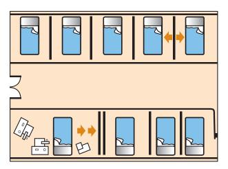
An example of a typical ward layout showing the versatility of Movatrack 101. Mobile tracks can be moved to instantly create more space around a bed.
