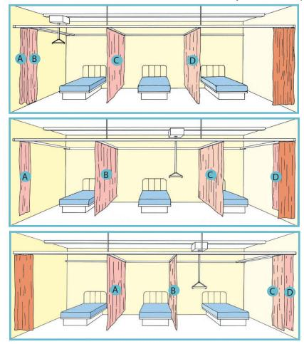
Many hospitals are struggling with the conflicting requirements of patient lifting hoists and cubicle curtain tracks. When a hoist track crosses a line of beds, as shown, the hoist itself or its apparatus is unable to pass over the cubicle track dividing rail. This is where Movatrack 101, with its mobile dividing rails, has the answer. In the illustration, A & B are two spare tracks, with curtains stacked at front of track. The hoist is parked over bed 1.
