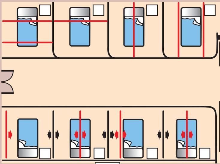
The traversing IV tracks of Movatrack IV400 Mobile are shown here in conjunction with Movatrack 101 Mobile cubicle track. The versatility of the system is immediately apparent, giving total flexibility of both bed space width and positioning of IV provision within it.
