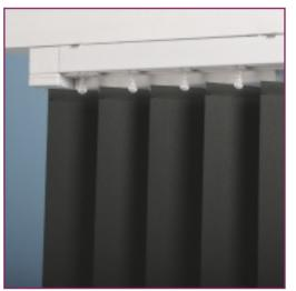
Features: 43 x 35mm white aluminium headrail with top-fix brackets and wheeled carrier trucks. A heavy-duty drive tape runs within the headrail, controlling both louvre tilt and draw, and powered by a 240v AC motor with individual switch control. 127/89mm louvres with weights and white stabilising chain
