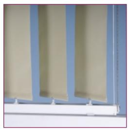
Features: Twin 28 x 27mm white aluminium ribbed headrails with face or topfix brackets and white carrier trucks. Metal bead-chain tilt control and cord draw, with controls looped between top and bottom tracks. 127/89mm louvres are held taut between tracks by sprung louvre hangers at top and bottom. Single or split draw.
