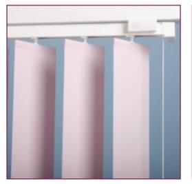
Features: 28 x 27mm white aluminium ribbed headrail with face or top-fix brackets and white carrier trucks. Draw operation is by standard cord control but louvre tilt is by battery-powered electric motor. This is controlled by a hand-held infra-red remote transmitter. 127/89/63mm louvres with weights and white stabilising chain. Single or split draw.
