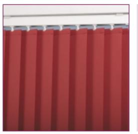
**Features:** 28 x 27mm white aluminium ribbed headrail with face or top-fix brackets and white carrier trucks. Draw operation is by drawing the control wand attached to the leading truck. Rotating the wand operates the louvre tilt mechanism. 127/89/63 louvres with weights and white stabilising chain. Optional VL21A has a 38 x 28mm profiled headrail.
